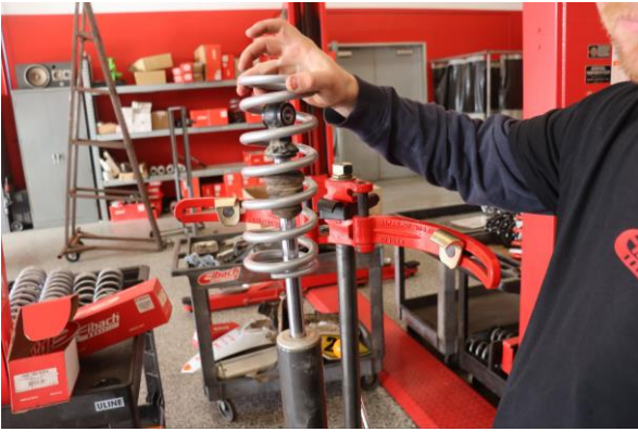
Install the Eibach secondary spring.
