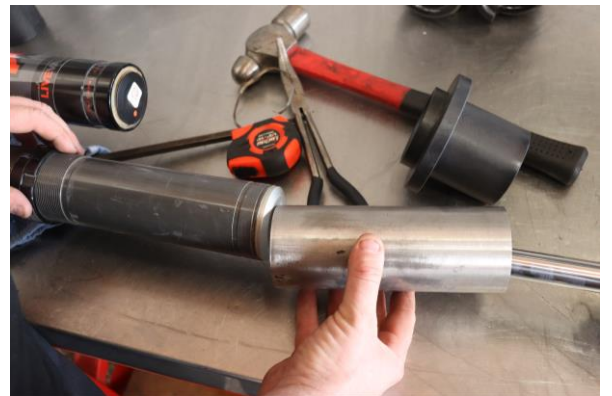
Remove the slider sleeve and crossover rings.
