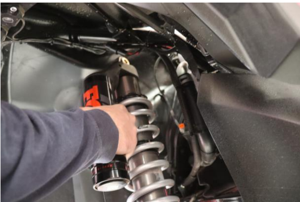
Re-install the coilover.
