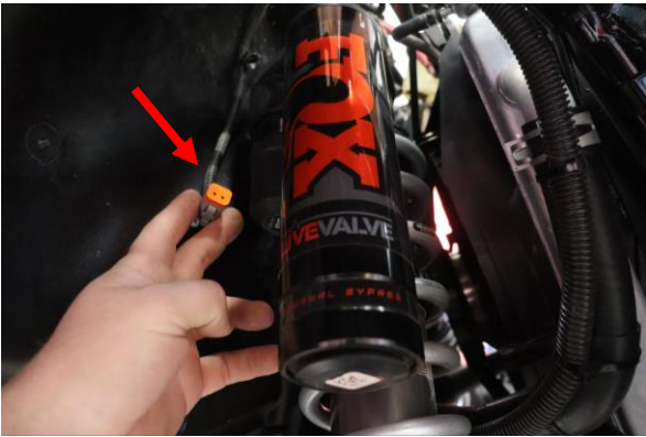
Disconnect the electrical connector at the top of the coilover.
