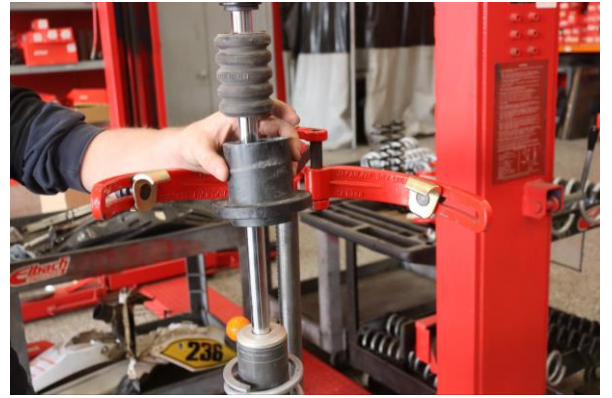
Remove OE spring slider.
