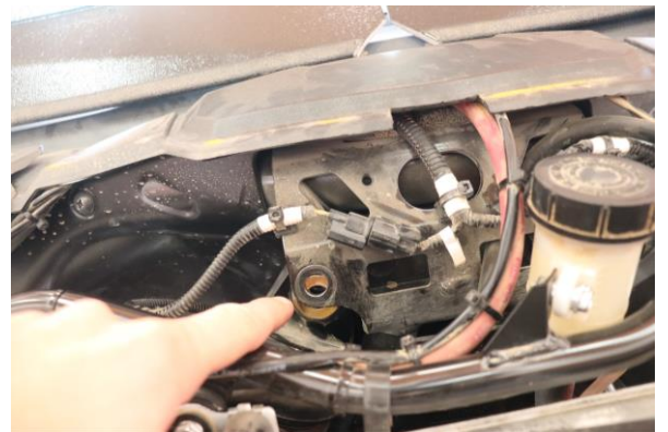
Secure the coilover to the upper mount with the OE hardware.
