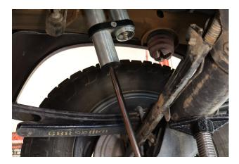
Reservoir should be mounted towards the top and pointing towards the axle on both sides of the vehicle.
