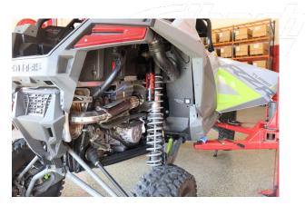
Reinstall the shock assembly and repeat on the opposite side. Torque shock bolts back to factory spec.
