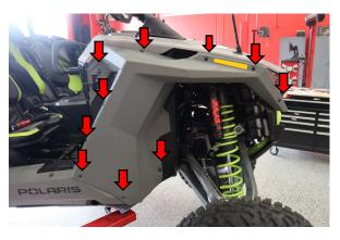
Remove the T40 torx bolts and clips on the fender and remove the fender.
