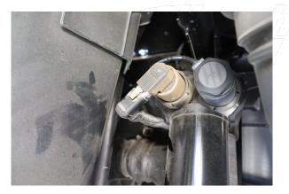
Unplug the harnesses for the Live Valve compression and rebound adjusters.
