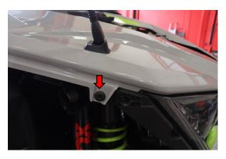
Remove the torx bolt on the side of the hood.
