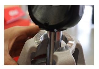
Install the OE lower spring perch. Make sure the perch is lined up with the boss on the clevis as shown.
