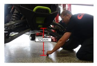
The front ride height should be about 525mm front the ground to the lower control arm bolt.
