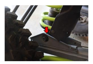
Remove the lower shock bolt with a 21mm wrench.
