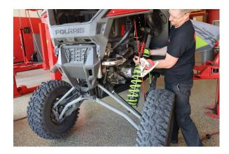
Remove the rear shock assembly.
