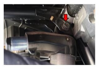
Remove the upper shock bolt with a 21mm wrench.
