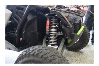
Repeat on the opposite side and reinstall everything in reverse order of removal. Torque shock bolts to factory spec.
