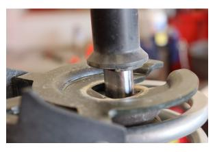
Compress the springs and install the OE lower spring perch. Make sure to align the boss on the rod end as shown.
