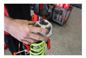
Compress the springs and remove the lower spring perch.
