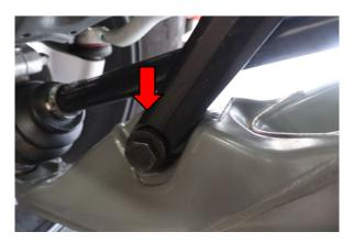
Loosen and remove the lower shock bolt with a 21mm wrench.
