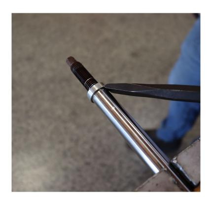
On both front and rear shocks remove this stem spacer from your OE shocks and transfer to your new Eibach shocks. Use of a hammer and punch may be necessary to remove.
