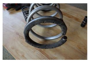
The bottom piece of tubing from the OE springs must be removed and installed on the Eibach springs.
