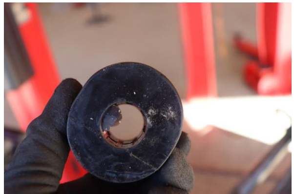
16. Add the supplied sway bar grease to the supplied bushings.
