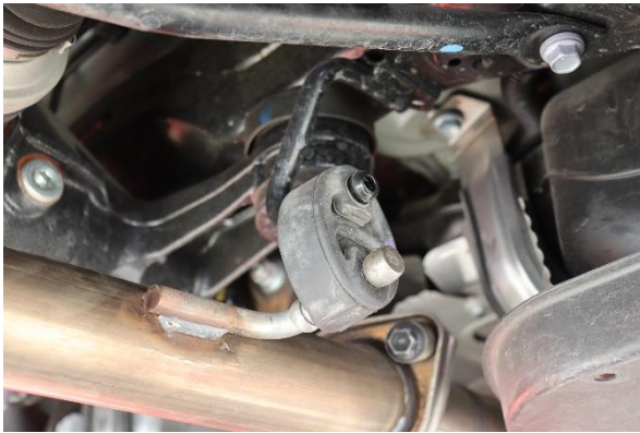
3. Remove both rubber exhaust hangers.
