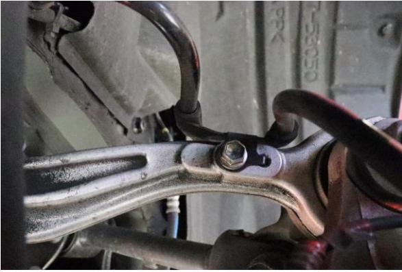
7. Remove the 10mm bolt for the brake line bracket.
