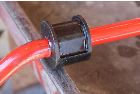
17. Install the lubricated bushing on the sway bar as shown.
