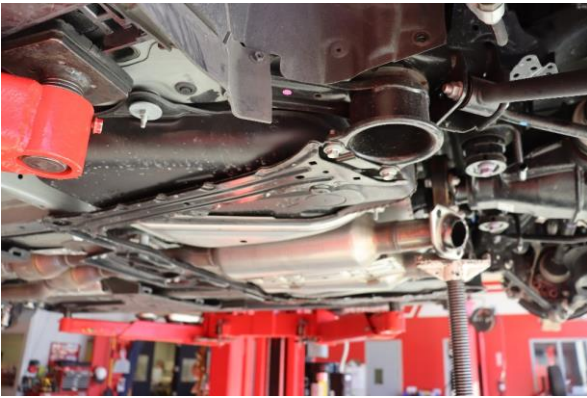
9. Remove the rear chassis brace.
