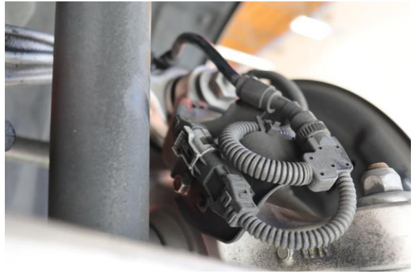
8. Remove the 10mm bolt for the wiring harness bracket.
