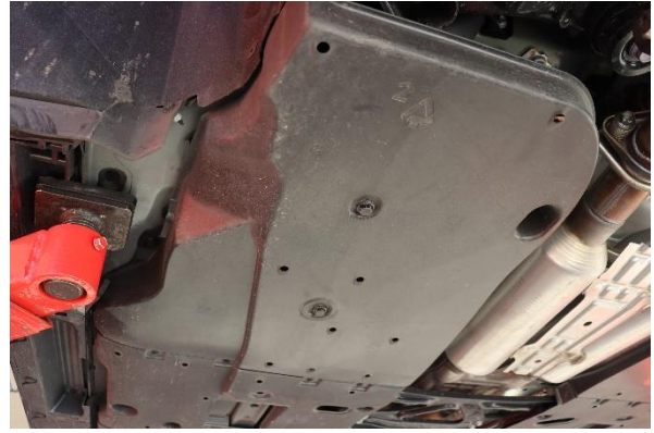
2. Remove the rear panels by pulling the plastic rivet clips, 10mm plastic nuts, and 8mm bolts.
