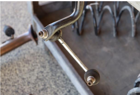
15. Remove the 17mm nut for the sway bar end links.
