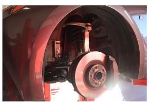
1. Safely lift vehicle and remove the front wheels.
