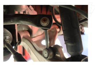
2. Remove the endlink nut with a 17mm socket.
