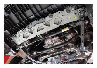
Reinstall the subframe reinforcement braces.
