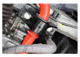
Using the OE bolts mount the Eibach bracket to the subframe.
