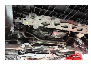
6. Loosen and Remove the OE sway bar brackets. With a 14mm socket
