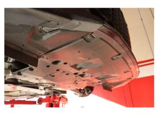
4. Remove the under tray with a 10mm socket and clip plyer to remove the plastic rivets.
