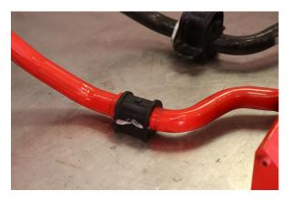
Install the bushings and brackets in the position as shown.
