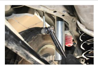
6. Disconnect the end link from the anti-roll bar as shown.
