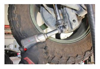
7. Loosen and remove lower shock bolt.
