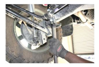
5. Use a screw or pole jack to support the rear axle as shown.
