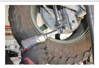
16. Secure the shock mount to the axle using the OE hardware as shown.
