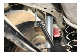
17. Reconnect the end link to the anti-roll bar with the OE hardware as shown.
