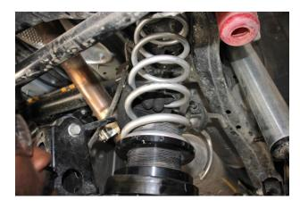
13. Pull down on the axle and install the supplied spring. Note: Do not stretch brake lines/ABS lines, or vent lines as this could cause failure of these components.
