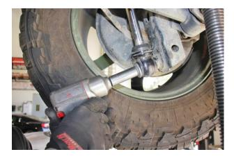
7. Loosen and remove lower shock bolt.
