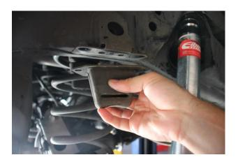
2. Loosen and remove the bolts that secure the OE bump stop to the chassis as shown, then, remove the bump stop.
