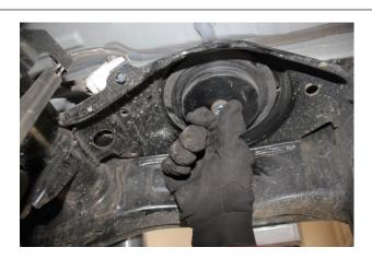
10. Install the provided spring perch adapter and secure it with the M12 x 1.75 x 30mm hex screw, and M12 washer/nut.
