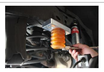
4. Install the new bump stop assembly using the M8  $\times$  1.25  $\times$  60mm bolts and M8 flat washers as shown.
