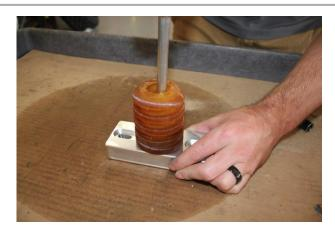
3. Use the M10 x 1.5 x 30mm bolts to secure the provided Eibach bump stop to the Eibach bump stop mount as shown.
