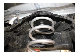
15. Ensure the spring is properly seated on the upper adapter, lower spring seat, and that the urethane adapter is seated correctly on the axle.
