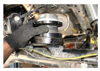
12. Install the adjustable spring perch assembly onto the urethane spring perch adapter on the axle as shown.
