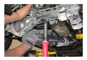
14. Compress the spring enough to install the lower mount of the shock to the axle.
