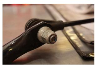
7. Remove the end link from the bar with a 15mm wrench
