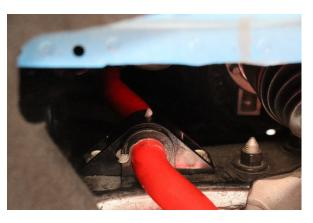
13. With the bar in the proper position install the provided brackets and secure them with the OE hardware using a 15mm socket.
