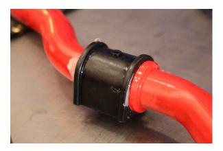
11. Install the bushings to the outside of the ring.
