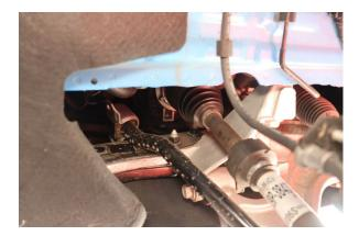
5. Remove the OE bar from the driver side of the vehicle.
