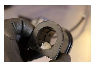
10. Apply the lubricant to the bushing
