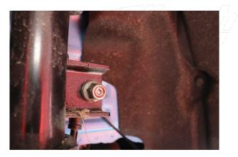
14. Reinstall the end link nut with a 18mm socket.
