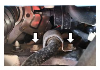
4. Remove the two bolts that secure the OE bar with a 15mm socket.
