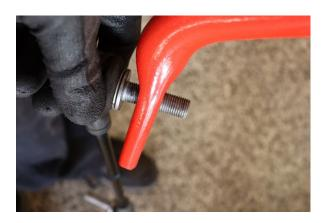
9. Attach the end links to the sway bar.
