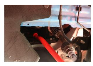
12. Install the bar with the end links and bushings installed.
