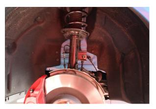
1. Properly lift and support the vehicle. Once secured removed the front wheels. The following procedure should be performed on both sides of the vehicle.
