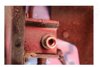
2. Remove the nut that secures the end link with an 18 mm socket.
