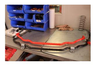
6. Confirm the orientation of the Anti Roll bar with the OE bar.
