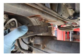
6. Safely lower the rear axle support and remove the stock lift block
