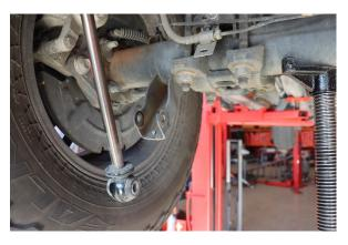
3. Swing the lower shock out of the opening on the rear axle
