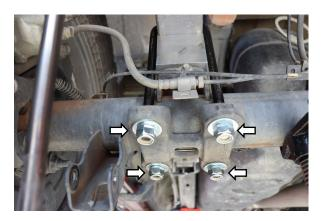
10. Secure the U-bolt bracket with the provided washers and 22mm nuts. Hand tighten each nut first so the u-bolts are showing equal threads on all sides.
