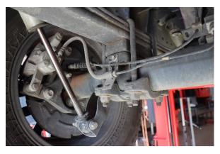
1. Start by lifting the vehicle and supporting the rear  $\mbox{\sc axle}$
