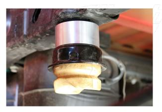
Install the lift block spacer on each side with the provided bolt. 2 different length bolts are provided depending on your vehicle.
