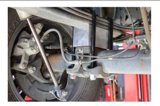
12. Reinstall the lower shock mount to the rear axle and repeat on the opposite side.
