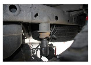
Loosen and remove the factory bump stops.
