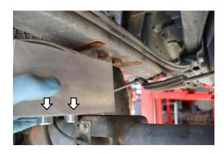
7. Install the Eibach 1.5" lift block with the pins facing the axle and the taper (shorter) end pointing towards the front of the truck
