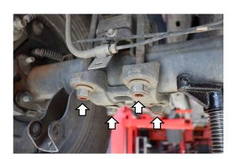
4. Remove the four 19mm nuts from the U-bolt bracket
