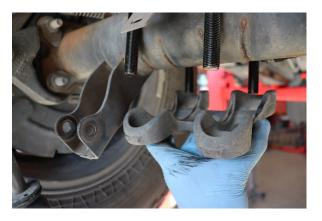
9. Reinstall the U-bolt bracket
