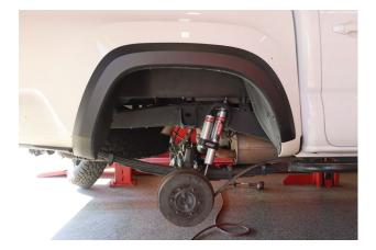
The reservoir should be mounted towards the top and pointing towards the back of the vehicle on both sides.
