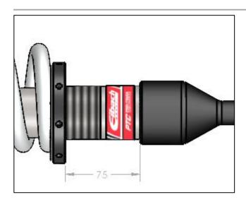
Note: Do **NOT** go above a spring perch height of 75mm or else damage to the shock and suspension will occur.
