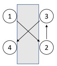
Tightening in a cross pattern is critical and failure to do so may result in suspension failure.
