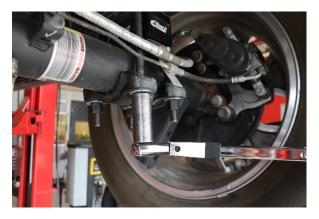
Tighten the u-bolts to 100 ft-lbs in a cross pattern shown to the right.
