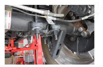
Reinstall the axle carrier and hand tighten the nuts equally before tightening with a wrench.
