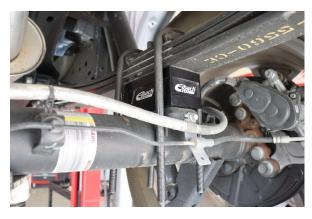
Raise the axle back up so the pins are fully seated on the top and bottom of the block and then reinstall the provided u-bolts.
