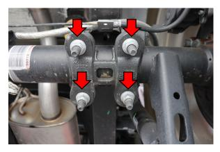
Loosen and remove the nuts at the bottom of the ubolts and the axle carrier.
