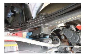
Lower the axle and remove the OE block. Make sure any brake lines or wires do not overstretch when lowering the axle.
