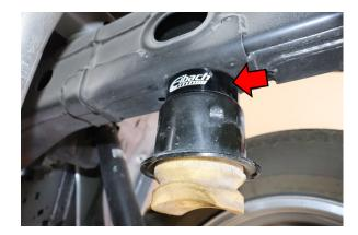
Install the provided bump stop spacer with the provided bolt.
