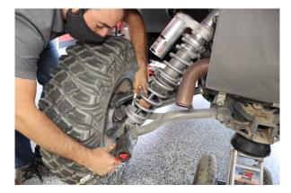
Step 16. Secure the coilover to the control arm with the OE hardware.
