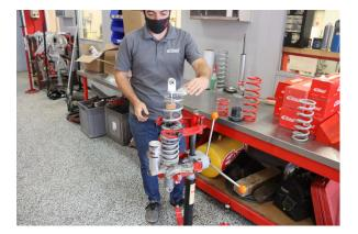
Step 13. Compress the spring assembly and reinstall the spring retainer.
