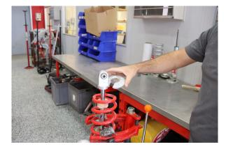
Step 4. Compress the coilover, then remove the spring retainer. Note: The bump stop will need to be pried down, out of the way of the spring retainer.
