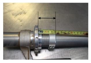
Step 9. Install the cross-over rings (8001224) and set them at **50mm** measuring from the spring flange to the bottom of the crossover ring.
