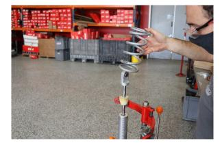
Step 10. Install the Eibach secondary spring (0800.300.0300S).
