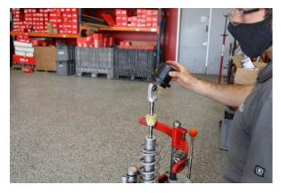
Step 11. Install the Eibach spring slider (8001100).
