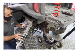
Step 14. Reinstall the coil over.
