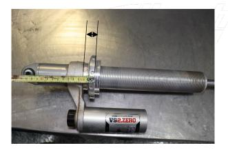
Step 8. Set the preload collar to **25mm** (FULL HIGH) measuring from the base of the reservoir housing to the spring flange.
