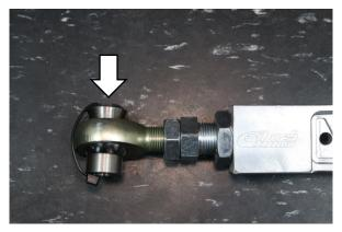
Before installing ensure that the tapered heim spacer is facing the knuckle of the vehicle.
