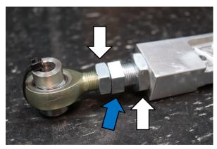
When making adjustments make sure the threads are equal by rotating from the center adjuster only. (Blue) DO NOT extend arm past 380mm eye to eye
