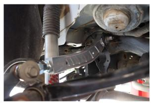
Step 2. Make sure that the adjustable arm is the same length eye hole to eye hole as the stock arm.
