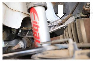
Step 3. Reinstall the wheel speed sensor wiring to the camber arm.
