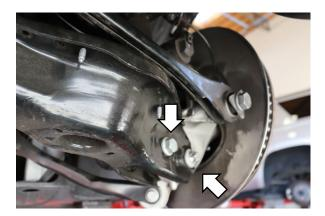
Reinstall the E20 and 18mm bolts for the lower control arm.
