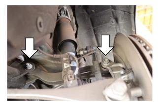
With the spring removed, you can now remove the two 18mm bolts for the OE camber arm.
