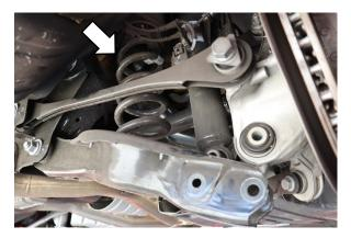
You can now pull down on the lower control arm and remove the spring.
