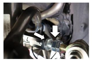
When adjusting the rear camber loosen the 24mm and 29mm jam nuts to adjust the rear camber of the vehicle. When the desired result is achieved lock the jam nuts back in place.
