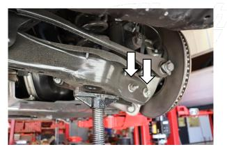
Support the lower control arm with a jack, then, remove the E20 bolt and 18mm nut. With the bolts completely removed lower the lower control arm.
