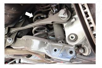
Reinstall the spring and support the lower control arm with a jack  $% \left( {{{\rm{A}}_{\rm{B}}}} \right)$
