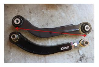
Set the Eibach Camber Arm to the same length as the OE camber arm before installation. Lock the jam nuts in positions once at the correct length. (This will be adjusted again later on an alignment rack.)
