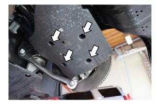
Reinstall the four 10mm nuts for the lower control arm cover
