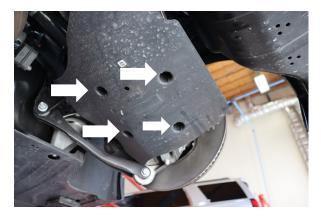
Remove the four 10mm nuts that secure the lower control arm skid plate.
