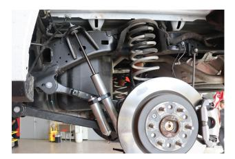
Reservoirs should be mount at the bottom and towards the front of the vehicle as shown.
