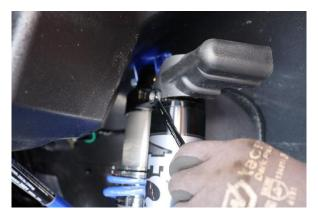
Step 2. Remove electrical connector cover from the top of the coilover.
