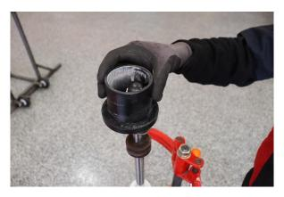
Step 14. Install the Eibach spring slider.
