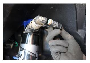
Step 3. Unplug electrical connector from the top of the coilover.
