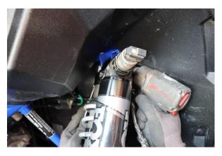
Step 19. Secure the coilover to the upper mount with the OE hardware.
