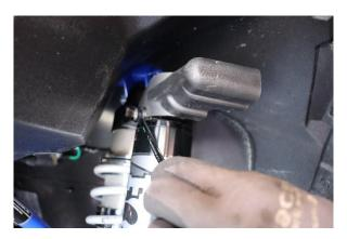
Step 22. Re-install electrical connector cover from the top of the coilover.
