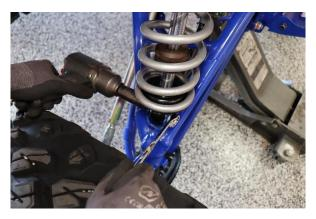
Step 20. Secure the coilover to the control arm with the OE hardware
