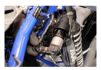
Step 22. Plug in the electrical connector at the top of the coilover.
