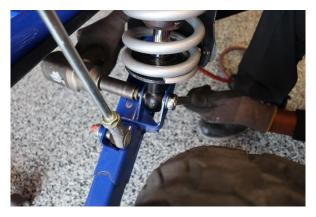
Step 20. Secure the coilover to the control arm with the OE hardware.
