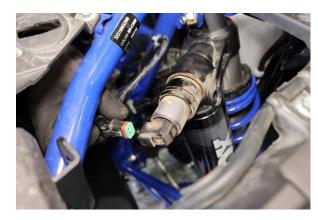
Step 5. Unplug electrical connector from the top of the coilover.
