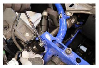
Step 21. Secure the coilover to the upper mount with the OE hardware.
