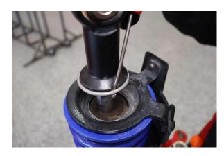
Step 6. Compress the coilover, remove the c-clip . Note: The bump stop will need to be pried down, out of the way of the spring retainer.
