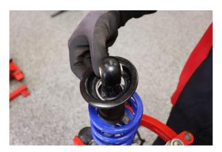
Step 8. Remove spring retainer.
