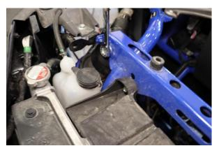
Step 3. Loosen and remove the hardware that secures the coilover to the upper mount.
