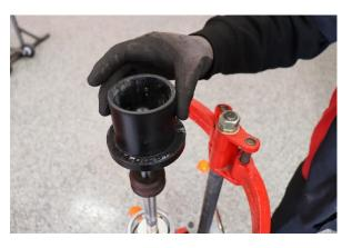
Step 15. Install the Eibach spring slider.
