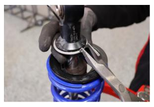
Step 7. Compress the coilover, remove the c-clip . Note: The bump stop will need to be pried down, out of the way of the spring retainer.
