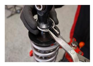
Step 18. Re-install C-clip. When releasing tension off of the spring assembly, make sure spring retainer fully seats on C-clip.
