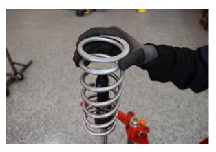
Step 13. Install the Eibach secondary spring.
