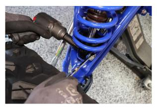
Step 2. Raise the front of the vehicle and support it with the proper safety equipment. Loosen and remove the hardware that secures the coilover to the control arm. Note: Never work on or under a vehicle that is not supported by the proper safety equipment.
