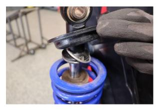
Step 7. Remove spring retainer.
