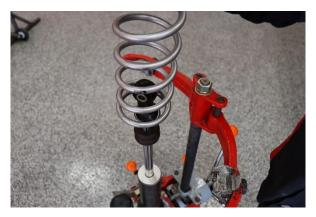
Step 14. Install the Eibach secondary spring.
