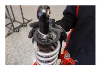
Step 16. Compress spring assembly and re-install spring retainer.
