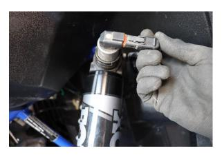
Step 21. Plug in the electrical connector at the top of the coilover.
