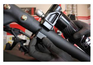
Step 23. Re-install resi one cage, fastened by the 4 socket head cap screws.
