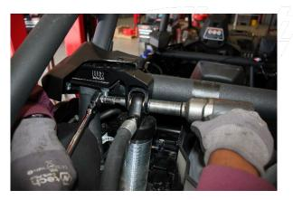
Step 2. Loosen hardware on the top mount, but do not remove the bolt.
