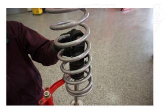
Step 14. Install the Eibach secondary spring.
