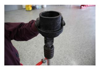
Step 15. Install the OE spring slider.
