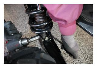
Step 1. Raise the rear of the vehicle and support it with the proper safety equipment. Loosen and remove the hardware that secures the coilover to the control arm. Note: Never work on or under a vehicle that is not supported by the proper safety equipment.
