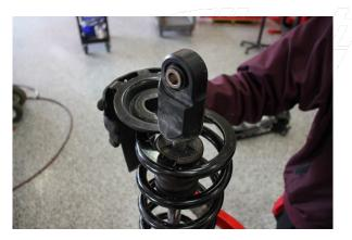
Step 8. Compress the OE spring assembly and remove the spring retainer. **Note: The bump stop will need to be pried down, out of the way of the spring retainer.**
