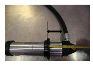
Step 12. Set the preload collar to **70mm** measuring from the base of the reservoir housing to the spring flange.
