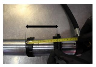
Step 13. Install the cross-over rings and set them at **125mm** measuring from the spring flange to the bottom of the crossover ring.
