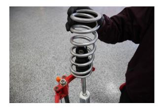
Step 11. Install the Eibach secondary spring.
