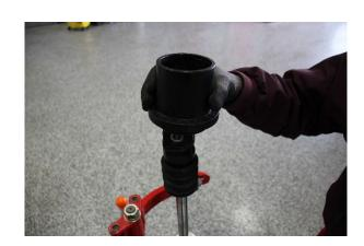
Step 12. Install the OE spring slider.
