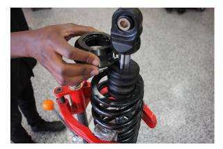
Step 5. Compress the coilover and remove the spring retainer. **Note: The bump stop will need to be pried down, out of the way of the spring retainer.**
