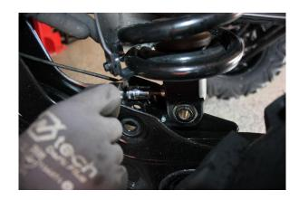
Step 6. Swing bottom of the shock out of the mounting clevis on lower control arm, remove two allen screws and pull electrical connector out of the bottom of the shock. Note: Be careful not to get dust/dirt inside of the electrical connector. Do not stretch wire as damage can occur.
