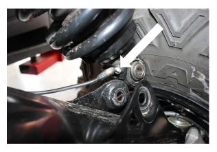
Step 3. Swing bottom of the shock out of the mounting clevis on lower control arm, remove two allen screws and pull electrical connector out of the bottom of the shock. **Note:** Be careful not to get dust/dirt inside of the electrical connector.
