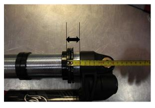
Step 9. Set the preload collar to **30mm** measuring from the base of the reservoir housing to the spring flange.
