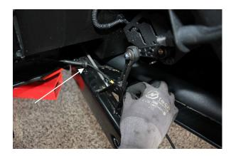
Step 5. Remove electrical wire from arm hold down to give enough slack to remove connector.
