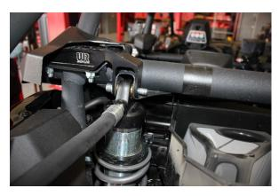
Step 19. Insert the bolt in the top mount, leave loose for now.
