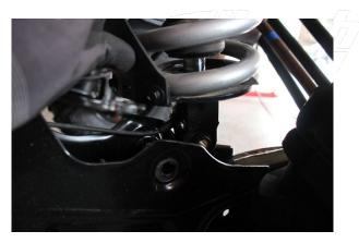
Step 20. Carefully plug the electrical connector back in at the bottom of the coilover, secure with OE allen screws. Note: There is a locater pin on the connector, ensure it is clocked properly. Do not over tighten connector.
