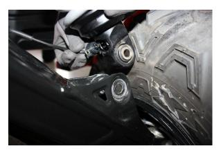
Step 17. Carefully plug the electrical connector back in at the bottom of the coilover, secure with OE allen screws. Note: There is a locater pin on the connector, ensure it is clocked properly. Do not over tighten connector.
