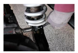
Step 22. Secure the coilover to the control arm with the OE hardware. Tighten upper mount hardware.
