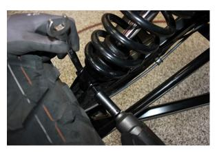
Step 1. Raise the front of the vehicle and support it with the proper safety equipment. Loosen and remove the hardware that secures the coilover to the control arm. Note: Never work on or under a vehicle that is not supported by the proper safety equipment.
