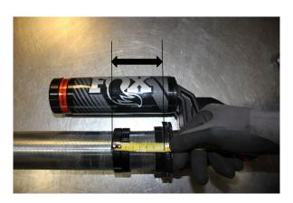
Step 10 . Install the cross-over rings and set them at **75mm** measuring from the spring flange to the bottom of the crossover ring.
