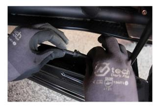
Step 4. Remove electrical wire from arm hold down to give enough slack to remove connector.
