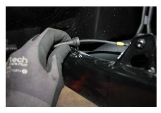
Step 21. Secure the wire to all mounting locations on the control arm.
