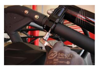
Step 3. Remove the 4 socket head cap screws fastening the resi to the cage. Place the resi in the bed.
