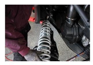
Step 18. Re-install the coilover. Carefully feed the resi/resi hose through the hole in the bed. Lay resi on the bed.
