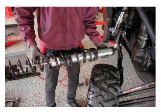
Step 7. Remove the bolt on the upper mount and remove the coilover.
