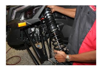
Step 4. Remove bolt from upper mount and remove coilover.
