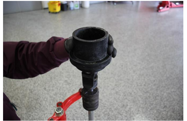
Step 10. Remove OE spring slider.
