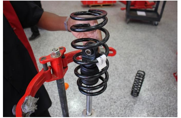
Step 8. Remove OE secondary spring.
