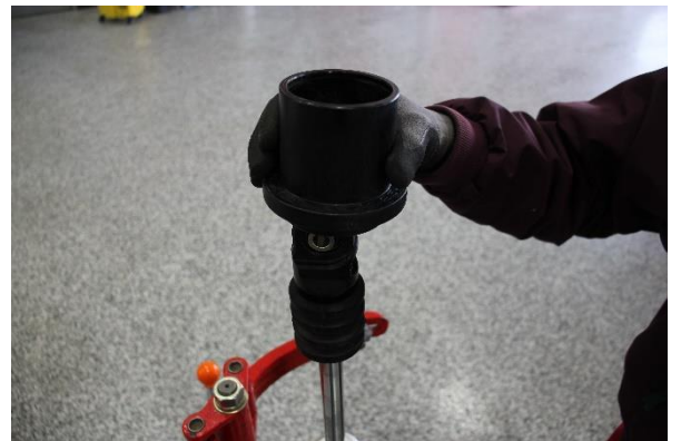
Step 12. Install the OE spring slider.
