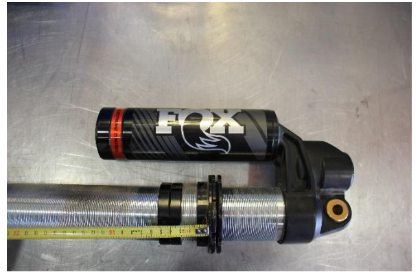
Step 10. Install the cross-over rings and set them at 55mm measuring from the spring flange to the bottom of the crossover ring.
