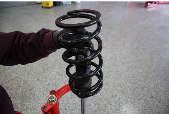
Step 11. Remove OE secondary spring.
