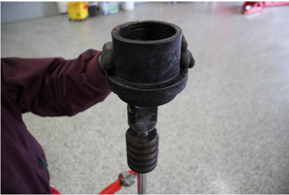
Step 15. Install the OE spring slider.
