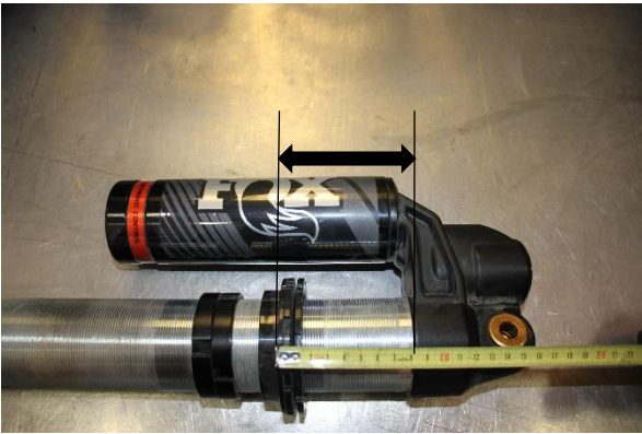
Step 9. Set the preload collar to 85mm measuring from the base of the reservoir housing to the spring flange.
