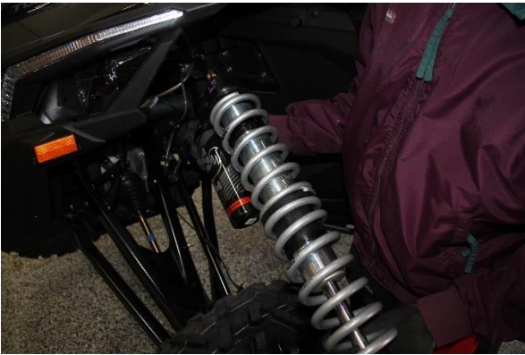
Step 15. Re-install the coilover.
