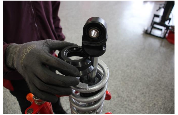
Step 14. Compress spring assembly and re-install spring retainer.
