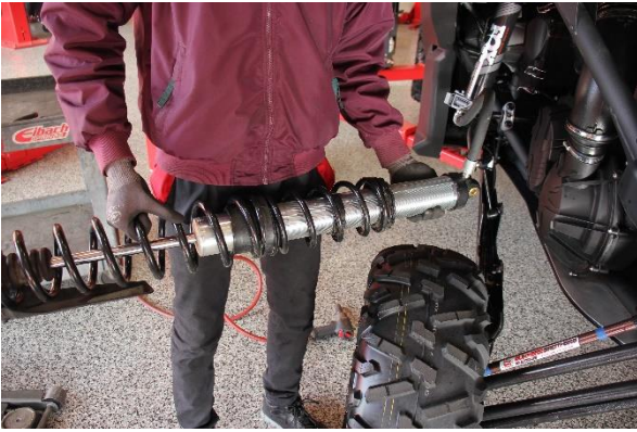
Step 7. Remove the bolt on the upper mount and remove the coilover.
