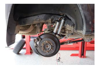
The reservoir should be mounted towards the top and pointing towards the axle on both sides of the vehicle.
