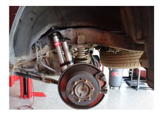
The driver and passenger shocks will have a different locating tab to orient the reservoir away from the frame. The locating tabs will be marked with a "D" or "P" to notate with side they belong on. The part number stamped on the shocks will also be marked. Failure to put the shocks on the correct side will cause issues fitting them to the vehicle and damage to your shock.
