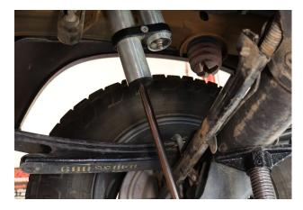
Reservoir should be mounted towards the top and pointing towards the axle on both sides of the vehicle.
