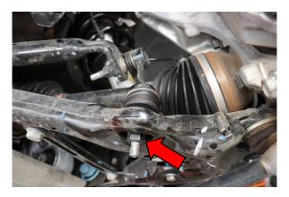
**Step 6:** Unbolt the 18mm nut for the sway bar end link. This will allow the lower control arm to droop more after the strut lower mounts have been removed.
