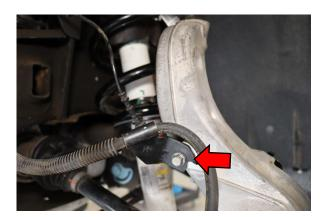
**Step 4:** Unbolt the 10mm bolt for the brake line bracket and remove the bracket
