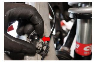
**Step 17:** Reinstall the bracket for the wheel speed senor into the steering knuckle using a 10mm bolt.
