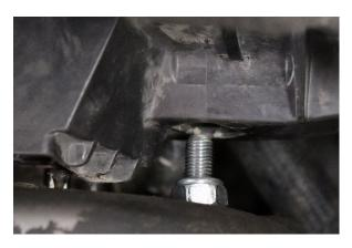
**Step 12:** Tighten the three flange nuts from the strut assembly top hat to the shock tower (43 ft-lbs).
