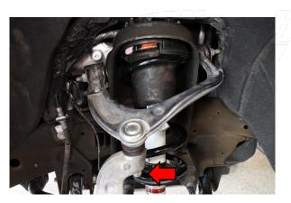
Step 8: Loosen, but do now remove the 18mm nut to separate the upper control arm from the steering knuckle. The upper control arm is preloaded and may swing upwards upon nut removal, use a pry bar to keep force applied to the UCA, remove the nut and slowly let the UCA swing up.
