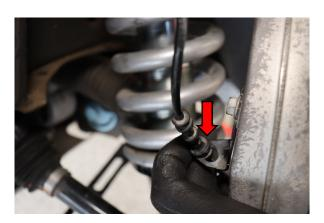
**Step 16:** Reinstall the wheel speed sensor grommet into the bracket
