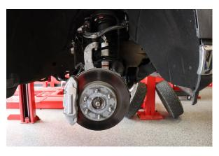
Step 1: Stock shock assembly that will be removed.
