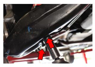
**Step 13:** Reinstall the 15mm bolts with the OEM brackets installed on the lower shock mount (37 ft-lbs).
