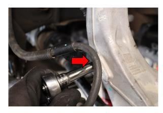
**Step 18:** Reinstall the brake line bracket into the steering knuckle by tightening the 10mm bolt.
