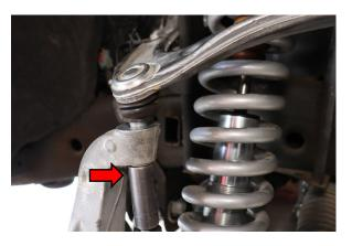
Step 15: Lower the Upper Control Arm into the steering knuckle. Note: The Upper Control Arm contains bushing preload and will need to be held in place using a pry bar. Once in the proper position secure the arm with the 18mm nut and tighten to 89 lb-ft then a 45-60 degree turn.
