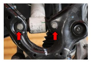
**Step 7:** Unbolt the 15mm bolts for the lower shock mounts. Be sure to remove the OE brackets on top of the lower mounts. You will install them on the Pro Truck Coilover 2.0.
