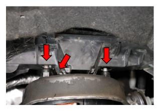
**Step 9:** Lift wiring harness off of the factory strut stud. Remove the three 18mm nuts for the upper strut mount located under the wiring harness bracket.
