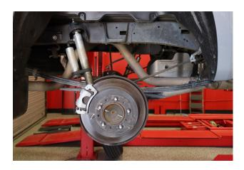
The reservoir should be mounted towards the top and pointing away from the axle on both sides of the vehicle.
