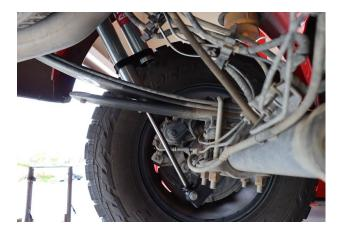
Reservoir should be mounted towards the top and pointing towards the axle on both side of the vehicle.
