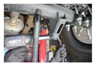
Reinstall the lower shock mount to the shock
