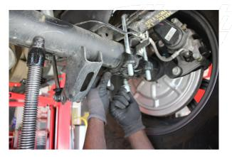
Install the provided washers and nuts and hand tighten so each end is even tightened. Do not tighten completely at this point.
