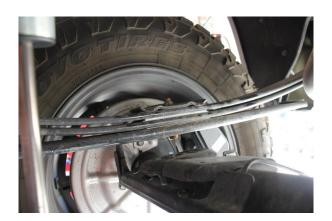
Lower the axle enough to insert the new lift block
