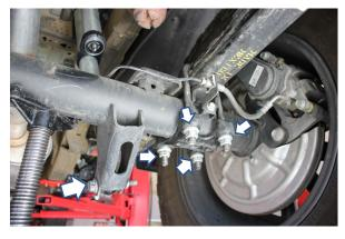
With the vehicle raised and properly supported loosen and remove the hardware securing the lower shock mount and the 4 nuts and U-bolts securing the axle to the leaf spring
