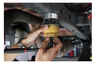
Remove the bolt securing the bump stop to the frame and reinstall with the provided bump stop spacer and longer bolt.
