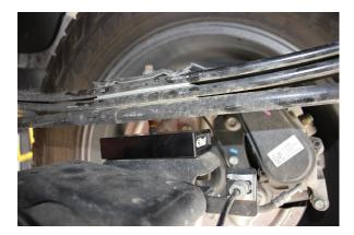
Insert the lift block with the pin pointing down located in the whole on the axle pad
