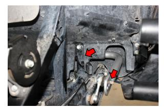
Loosely reinstall the plate and end links and make sure everything fits correctly.
