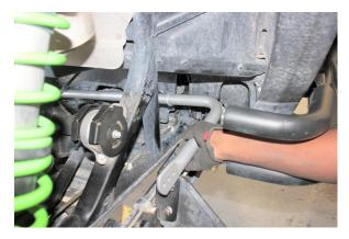
Install the Eibach sway bar in the same orientation as the stock bar.
