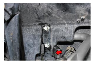
Reinstall the screw holding the plastic cover and road test the vehicle. After road testing the vehicle check again to make sure all the bolts are still tight.
