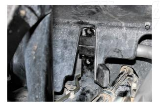
Make sure the new bushings are properly installed into the opening in the frame.
