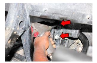
Loosen and remove the bolts holding the plate onto the sway bar bushing.
