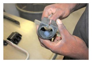
Lubricate the new bushings with the provided grease before installing on the Eibach sway bar.
