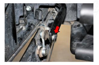
Loosen and disconnect the end link from the sway bar.
