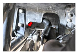
Begin by removing the screw holding the plastic to the frame near the bracket on both sides.
