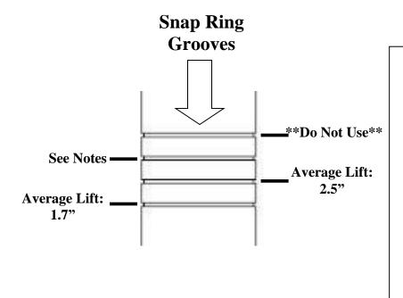
**Important:** Ensure that the snap ring is fully seated in the snap ring groove (you should be able to rotate the snap ring manually/by hand). **Note: Improper installation will cause permanent damage to the shock. Please refer to the Pro Truck Sport Damper instructions for more info regarding proper installation and fitment.**
