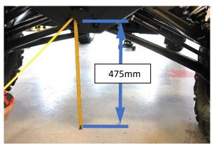
Step 18. The recommended preload measurement in **Step 9** will get the vehicle close to the recommended ride height but each vehicle may vary some. We recommend setting the ride height at 480mm measuring from the ground to the center of the lower control arm bolt. Shock eye to eye length should be about 730mm **Note: These measurements were on a 30in tire size if you have larger than stock wheels and tires, the ride height will be increased.**
