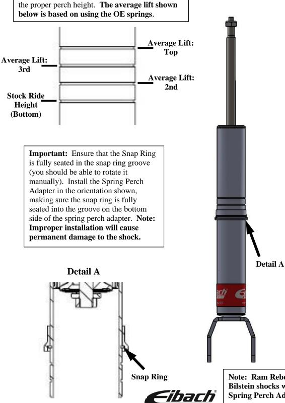
Note: If using the Eibach Pro Lift springs, refer to the instructions for the Eibach springs to determine
