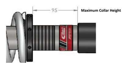
Note: Do NOT go above a spring collar height of 95mm from bottom of collar to base, as shown or else damage to the shock and suspension will occur.
