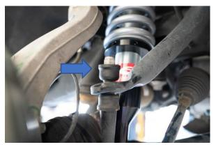
Step 19. Re install the end link and tighten 15mm nut to (22 ft-lb)
