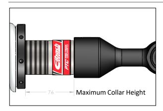
Note: Do NOT go above a spring collar height of 76mm from bottom of collar to base, as shown or else damage to the shock and suspension will occur.
