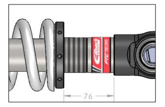
Not: Do **NOT** go above a spring perch height of 76mm or else damage to the shock and suspension will occur.
