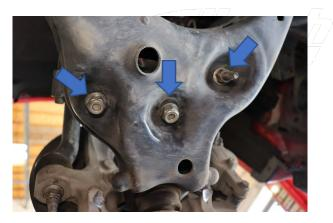
Step 7. Remove the shock assembly lower nuts.
