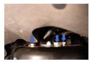
Step 12. Install the 3 flange nuts provided with the kit to the top hat on shock tower.
