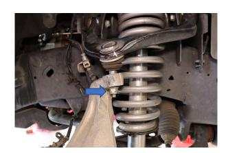
Step 5. Separate the ball joint from the knuckle.
