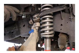
Step 15. Use a pry bar to ease the upper control arm down into the spindle and fasten the nut on the bottom.
