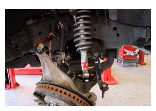
Step 10. Press downward on the lower control arm and remove the strut assembly.
