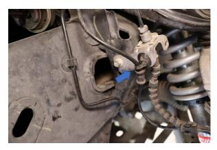
Step 16. Reattach the wheel speed sensor to the upper brake hose bracket.
