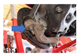
Step 3. Remove the tie-rod nut and disconnect the tie-rod from the knuckle
