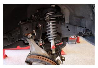
Step 6. Secure the spindle so that there is no tension in the brake line.
