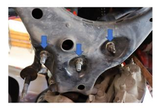
Step 13b. Fasten lower shock nuts
