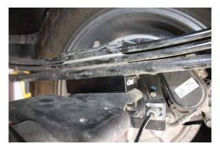
Raise the axle so the locating pin on the bottom of the leaf springs is located in the hole on the top of the lift block
