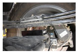
Insert the lift block with the pin pointing down located in the whole on the axle pad
