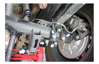
With the vehicle raised and properly supported loosen and remove the hardware securing the lower shock mount and the 4 nuts and U-bolts securing the axle to the leaf spring
