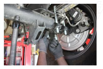
Install the provided washers and nuts and hand tighten so each end is evenly tightened. Do not tighten completely at this point.
