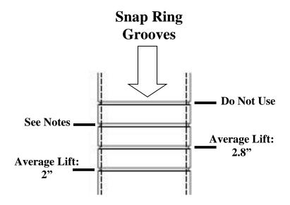
**Important:** Ensure that the snap ring is fully seated in the snap ring groove (you should be able to rotate the snap ring manually/by hand). **Note: Improper installation will cause permanent damage to the shock. Please refer to the Pro Truck Sport Damper instructions for more info regarding proper installation and fitment.**
