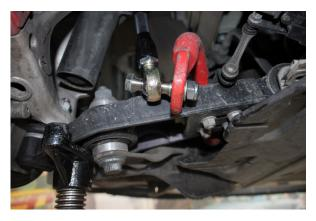
Install and secure the end link to the strut and the opposite end to the anti roll bar using the provided hardware as shown.
