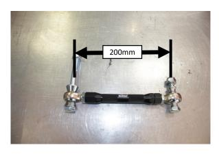
Adjust the Eibach end link to **200mm** from center to center as shown.
