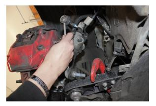
Make sure the lower control arm is supported by a floor or screw jack, then, loosen and remove the OE hardware that secures the OE end link to the end of the anti roll bar and the strut, then, remove the end link.
