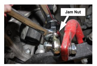
With the hardware properly secured, make sure the ends are properly orientated, then, tighten the upper and lower jam nuts.
