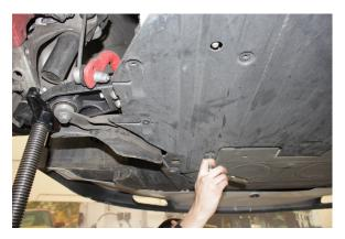
Begin by raising the vehicle and supporting it with the proper safety equipment, then, remove the front wheels. Note: Never work on or under a vehicle that is not supported by the proper safety equipment.
