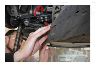
Loosen and remove the screws that secure the underbody cover as this will give you good clearance to access the lower end link hardware. (See Photos 1 & 2)
