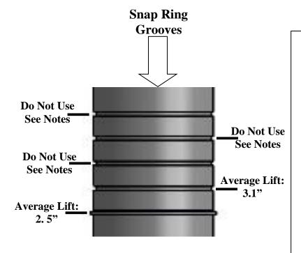
Important: Ensure that the snap ring is fully seated in the snap ring groove (you should be able to rotate the snap ring manually/by hand). Note: Improper installation will cause permanent damage to the shock. Please refer to the Pro Truck Sport Damper instructions for more info regarding proper installation and fitment.
