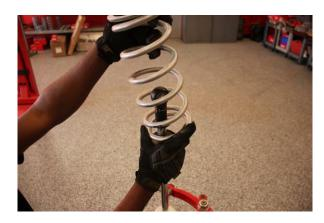
Step 12. Install the Eibach secondary spring.
