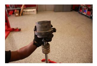
Step 13. Install the OE spring slider.
