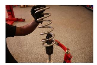
Step 10. Install the Eibach secondary spring.
