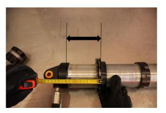
Step 10. Set the preload collar to **100mm** measuring from the base of the reservoir housing to the spring flange.
