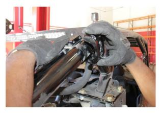
Step 19. Re-install the resi mounting bracket, secured by the 4 socket head cap screws.
