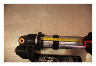
Step 9. Move the OE cross-over rings and set them at **80mm** measuring from the spring flange to the bottom of the crossover rings.
