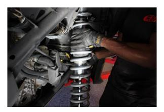
Step 16. Re-install the coilover, carefully guiding the resi back up through the hole in the bed.
