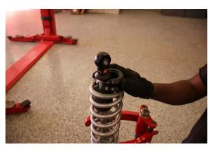
Step 13. Compress the spring assembly and reinstall the spring retainer.
