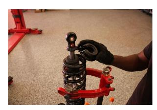
Step 4. Compress the coilover, then remove the spring retainer. **Note: The bump stop will need to be pried down, out of the way of the spring retainer.**
