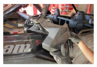
Step 20. Re-install the plastic cover fastened by 2 T30 screws.
