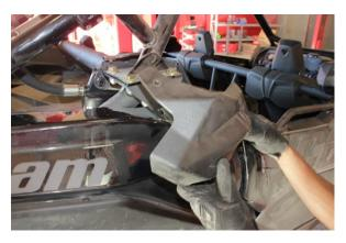
Step 1. Raise the rear of the vehicle and support it with the proper safety equipment. Remove the two T30 torx screws then remove the plastic cover. **Note: Never work on or under a vehicle that is not supported by the proper safety equipment.**
