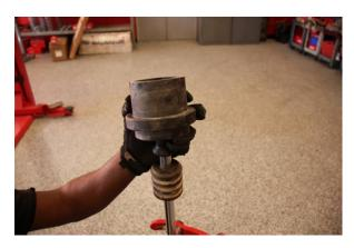
Step 13. Install the OE spring slider.
