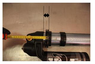
Step 8. Set the preload collar to **25mm** measuring from the base of the reservoir housing to the spring flange.
