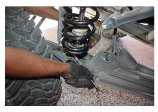
Step 3. Loosen and remove the hardware that secures the coilover to the control arm.
