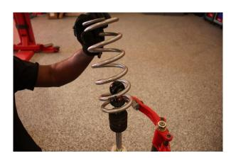
Step 10. Install the Eibach secondary spring.
