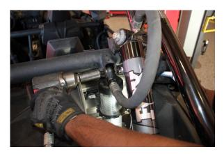
Step 4. Loosen and remove the hardware that secures the coilover to the upper mount.
