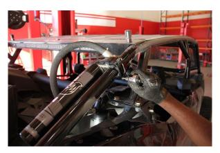
Step 2. Remove the 4 socket head cap screws on the resi mounting bracket, set resi in bed.
