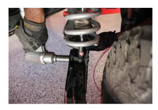
Step 18. Secure the coilover to the control arm with the OE hardware.
