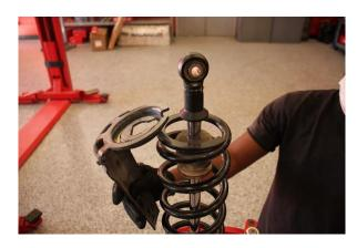
Step 6. Compress the coilover, then remove the spring retainer. Note: The bump stop will need to be pried down, out of the way of the spring retainer.
