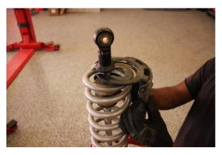
Step 15. Compress the spring assembly and reinstall the spring retainer.
