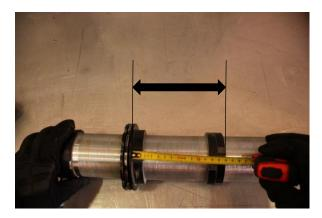
Step 11. Install the cross-over rings and set them at **140mm** measuring from the spring flange to the bottom of the crossover rings.
