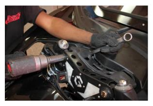
Step 16. Secure the coilover to the upper mount with the OE hardware.
