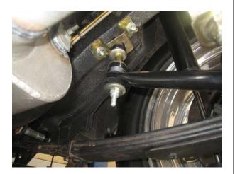
13. You can now rotate the end links brackets upwards and secure them to the U-Bolts with the provided hardware as shown. (See Photos 23 & 24)
