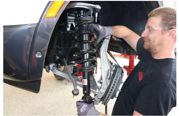
10. Remove the shock assembly from the vehicle.
