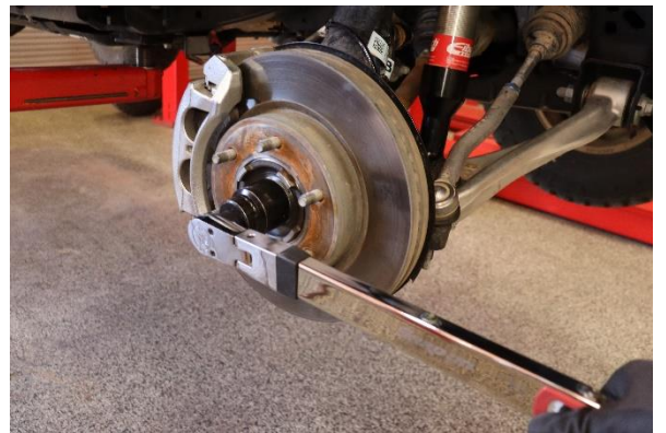
24. Reinstall the axle nut and torque to 221 ft-lbs.
