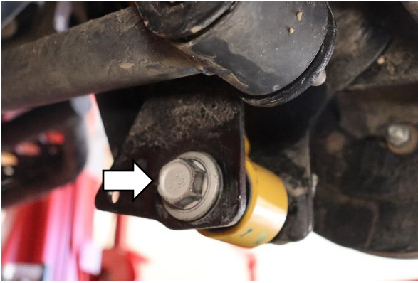
6. Safely support the rear axle and remove the lower shock mounting bolt with a 27mm socket.
