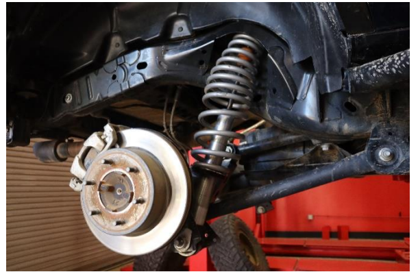
9. Install the rear coilover.
