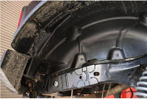
12. Place the fender liner back in the wheel well.
