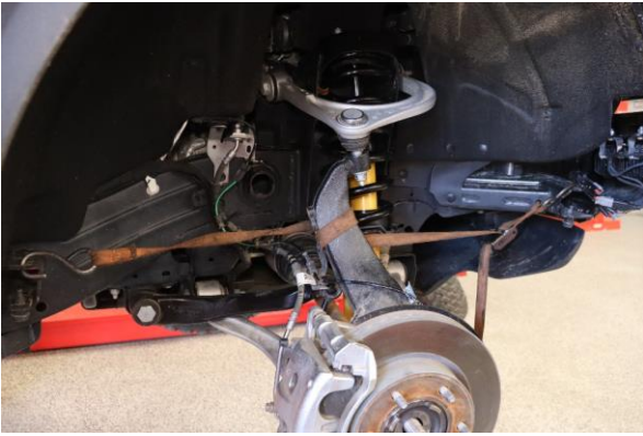
7. Strap the knuckle to prevent excessive droop and possible axle damage.
