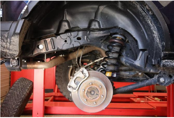
Rear Coilover Install
