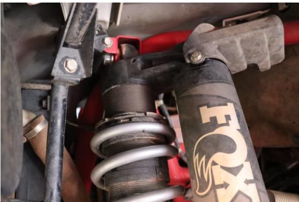
Step 23. Re-install electrical connector cover from the top of the coilover.
