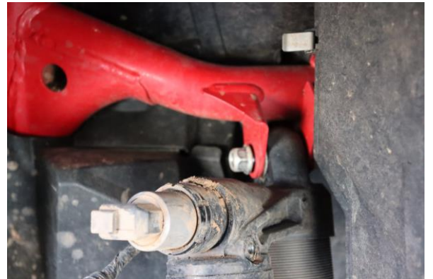
Step 4. Loosen and remove the hardware that secures the coilover to the upper mount.
