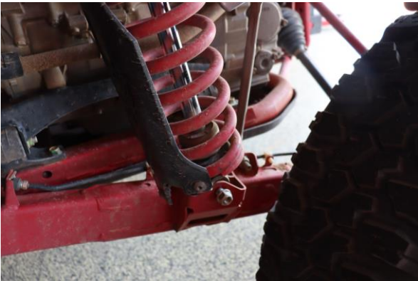
Step 3. Raise the rear of the vehicle and support it with the proper safety equipment. Loosen and remove the hardware that secures the coilover to the control arm. Note: Never work on or under a vehicle that is not supported by the proper safety equipment.
