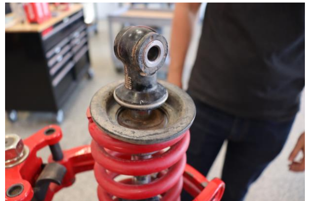
Step 6. Compress the coilover.
