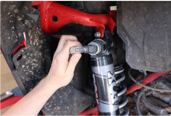
Step 21. Plug in the electrical connector at the top of the coilover.
