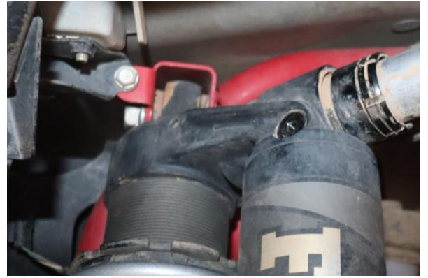
Step 20. Secure the coilover to the upper mount with the OE hardware.
