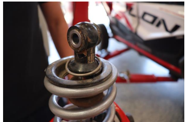
Step 18. Re-install C-clip. When releasing tension off the spring assembly, make sure spring retainer fully seats on C-clip.
