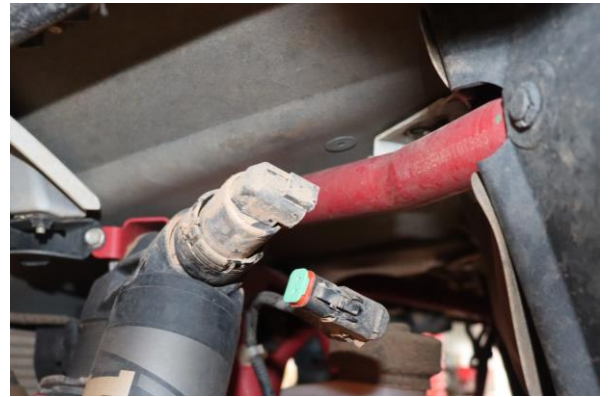
Step 22. Plug in the electrical connector at the top of the coilover.
