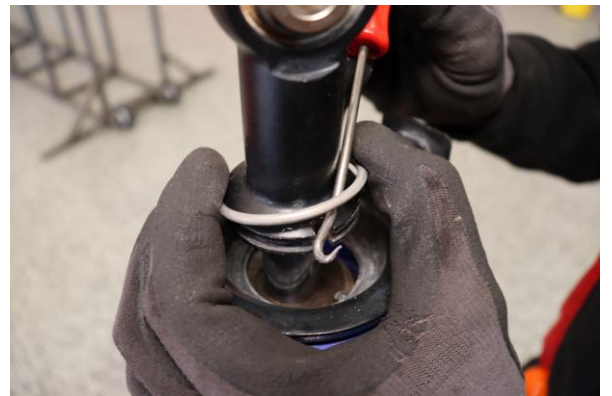
Step 6. Remove the c-clip. Note: The bump stop will need to be pried down, out of the way of the spring retainer.
