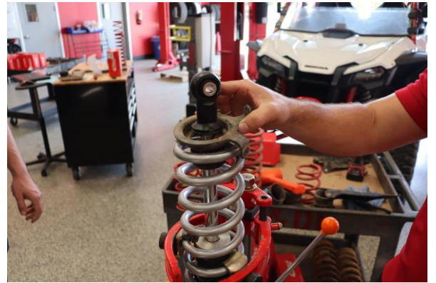
Step 16. Compress the spring assembly and re-install the spring retainer.
