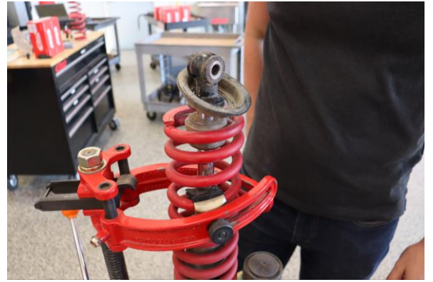
Step 8. Remove the spring retainer.
