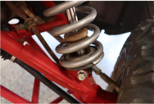
Step 21. Secure the coilover to the control arm with the OE hardware.
