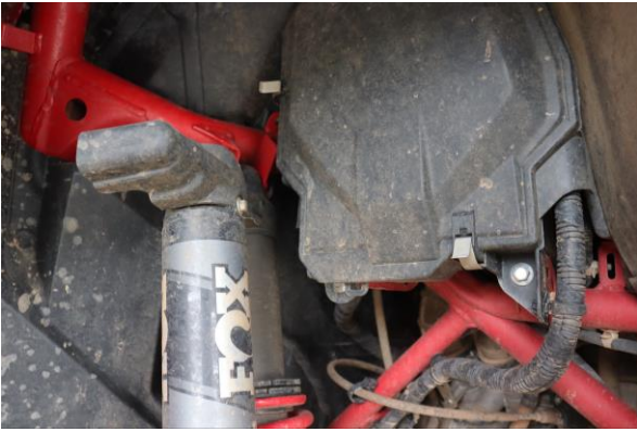
Step 1. Remove electrical connector cover from the top of the coilover.
