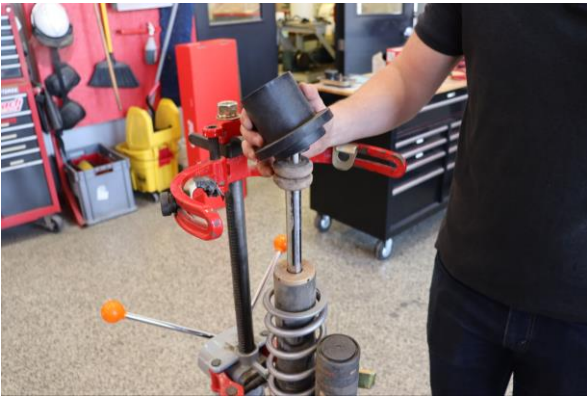
Step 15. Install the Eibach spring slider.
