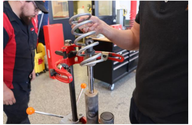
Step 14. install the Eibach secondary spring.
