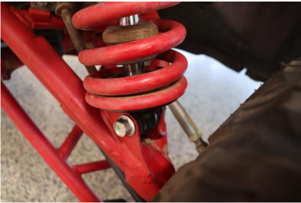
Step 3. Raise the front of the vehicle and support it with the proper safety equipment. Loosen and remove the hardware that secures the coilover to the control arm. Note: Never work on or under a vehicle that is not supported by the proper safety equipment.
