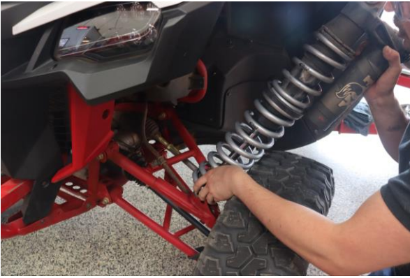
Step 19. Re-install coilover.
