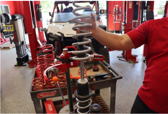
Step 15. Install the Eibach main spring.
