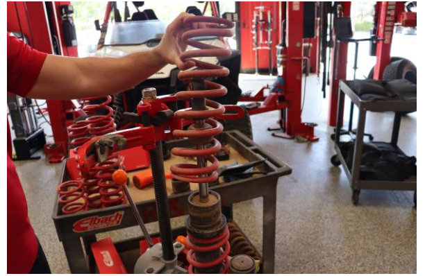
Step 8. Remove the OE main spring.
