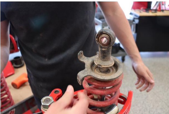
Step 5. Compress the coilover.
