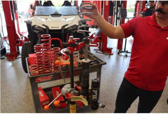
Step 13. Install the Eibach secondary spring.
