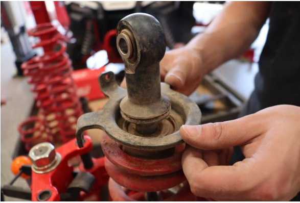
Step 7. Remove the spring retainer.
