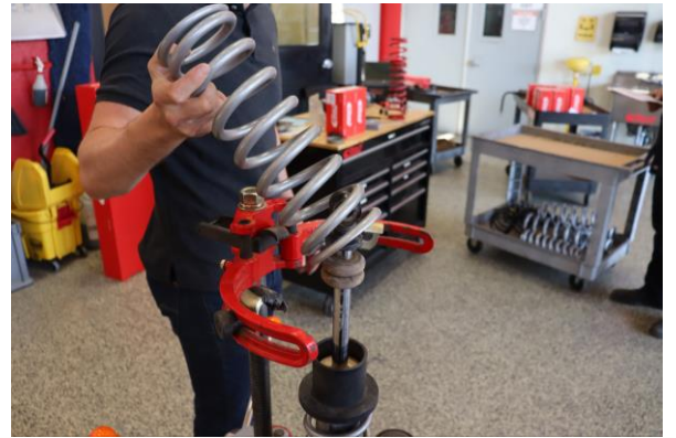
Step 16. Install the Eibach main spring.
