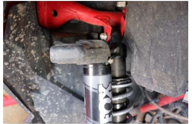
Step 22. Re-install electric connector cover from the top of the coilover.
