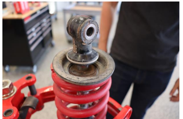
Step 6. Compress the coilover.
