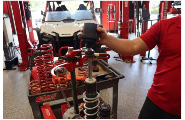
Step 14. Install the Eibach spring slider.
