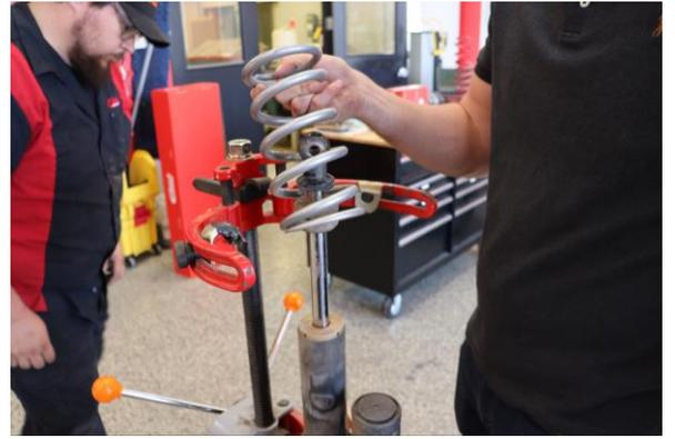
Step 14. install the Eibach secondary spring.
