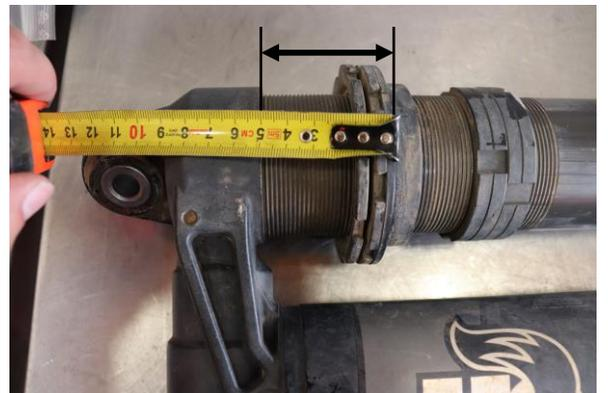
Step 12. Set the preload collar to **65mm** measuring from the base of the reservoir housing to the spring flange.
