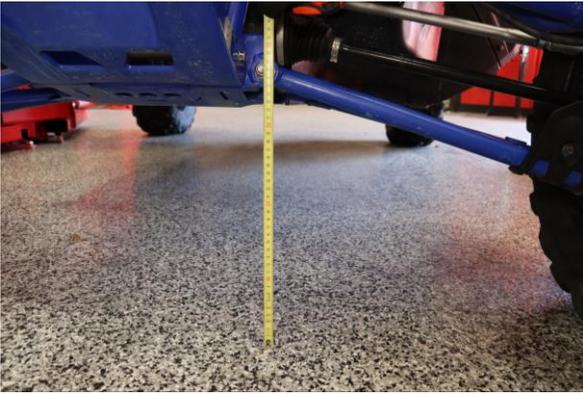
Step 24. Measure from the ground to the center of the lower control arm bolt. The recommended preload measurement in **Step 12** will get the vehicle close to the recommended ride height but each vehicle may vary some. We recommend setting the ride height at **390mm** measuring from the ground to the center of the lower control arm bolt. **Note: If you have larger than stock wheels and tires, the ride height will be increased.**
