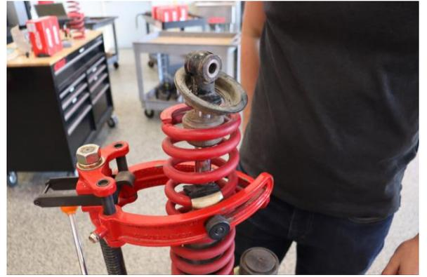
Step 8. Remove the spring retainer.
