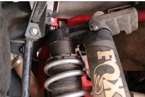
Step 23. Re-install electrical connector cover on the top of the coilover.
