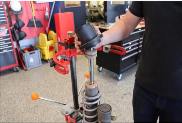
Step 15. Install the Eibach spring slider.
