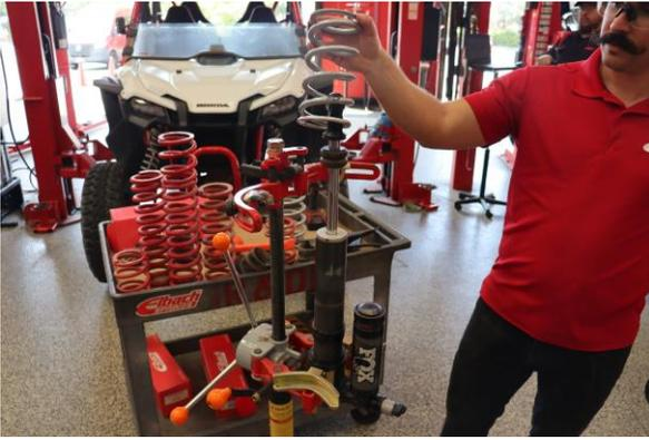
Step 13. Install the Eibach secondary spring.
