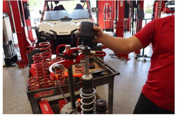
Step 14. Install the Eibach spring slider.
